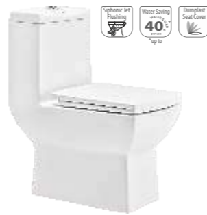
CLAYTON 220 Snow White 650 x 365 x 765 mm Cat. No. S1013203 S Trap 220 mm with duroplast soft close seat cover ₹ 18,490
